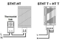
Model with T at the end of the code are fitted with fixed set point compact thermostat. Set is fixed at 5°C: the heating element starts to heat at enclosure temperature under 5°C and then it turns off at enclosure temperature higher than 15°C
